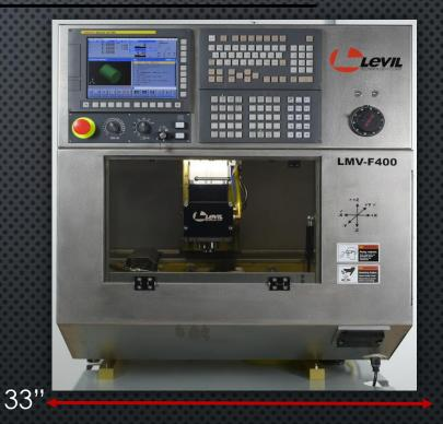
Resolution 0.00004" (0.001mm) Repeatability 0.0002" (0.005mm) Accuracy 0.0004" (0.01mm) Rapid Feed (X, Y & Z) 400 ipm (10,200 mm/min) Cutting Feed (X, Y & Z) 240 ipm (6,120 mm/min) Rapid Feed (4th Axis) 19 rpm (7,000 deg/min)
