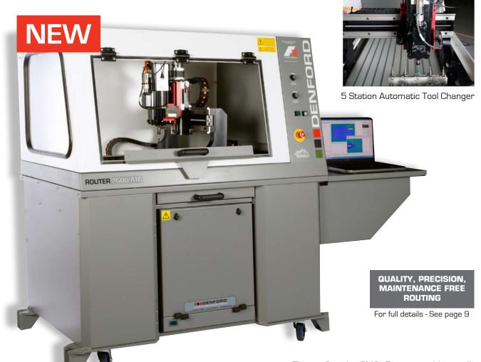
Router 2600 ATC shown with optional universal bench, optional computer support extension and optional integrated Dust Pro 100 (PC not included)
