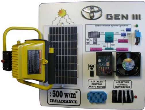
MEG-SV HVAC Automotive Solar Ventilation Trainer
