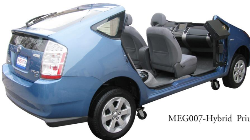
MEGART-PRIUS Prius Engine Cutaway
